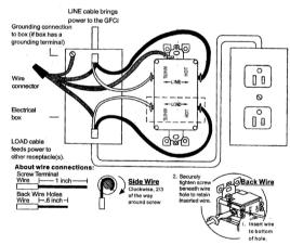
copper (or green) wire directly to the grounding terminal on the GFCI receptacle.
